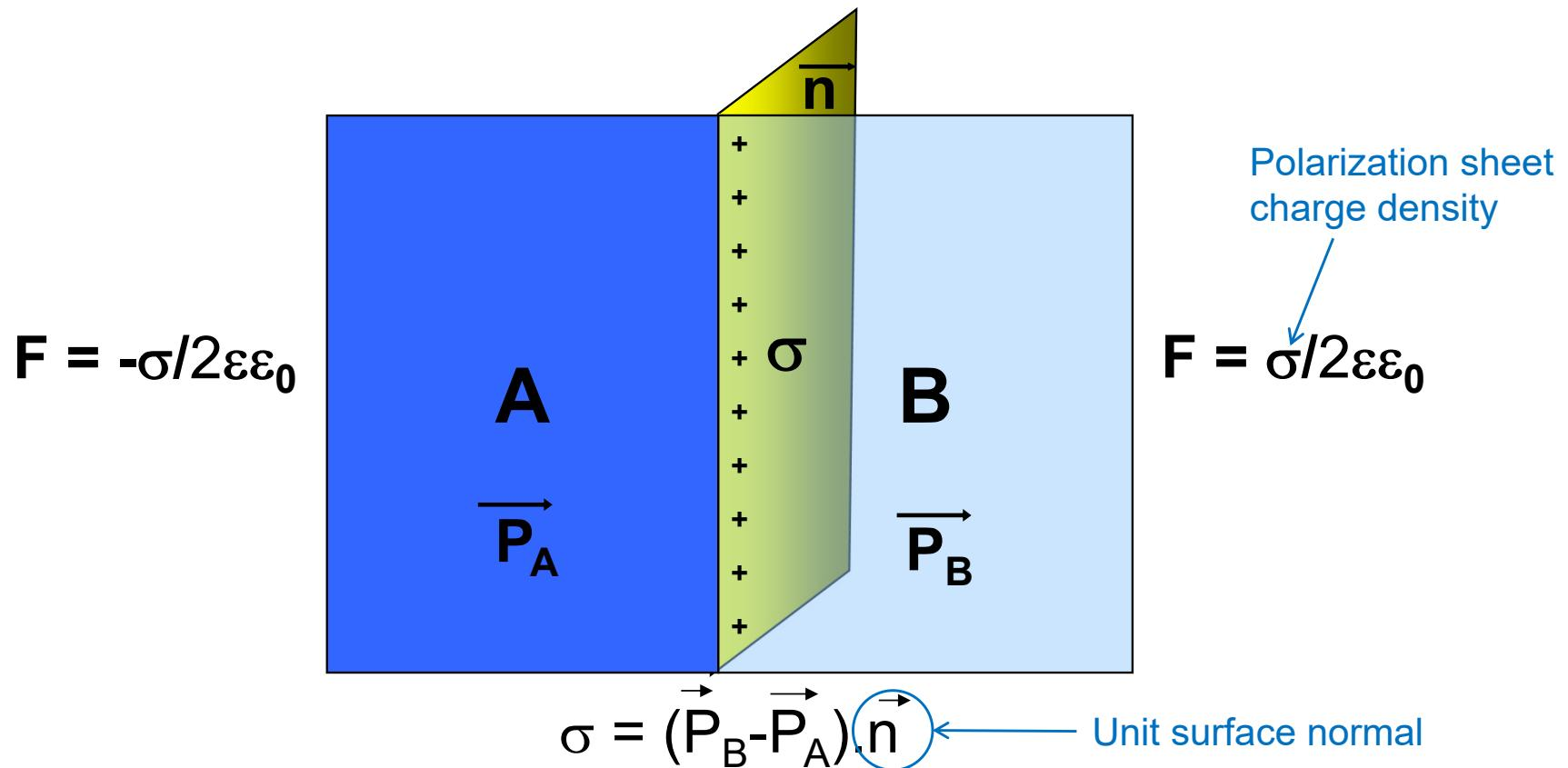
Spontaneous and piezoelectric polarization discontinuities at heterointerfaces
