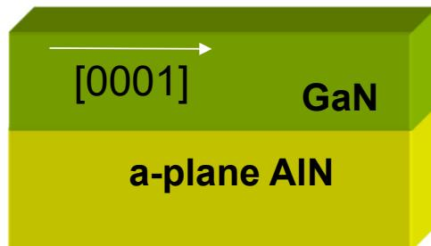
Growth on non-polar substrates  $\Rightarrow$  macroscopic polarization // QW plane  $\Rightarrow$  no fixed charge plane
