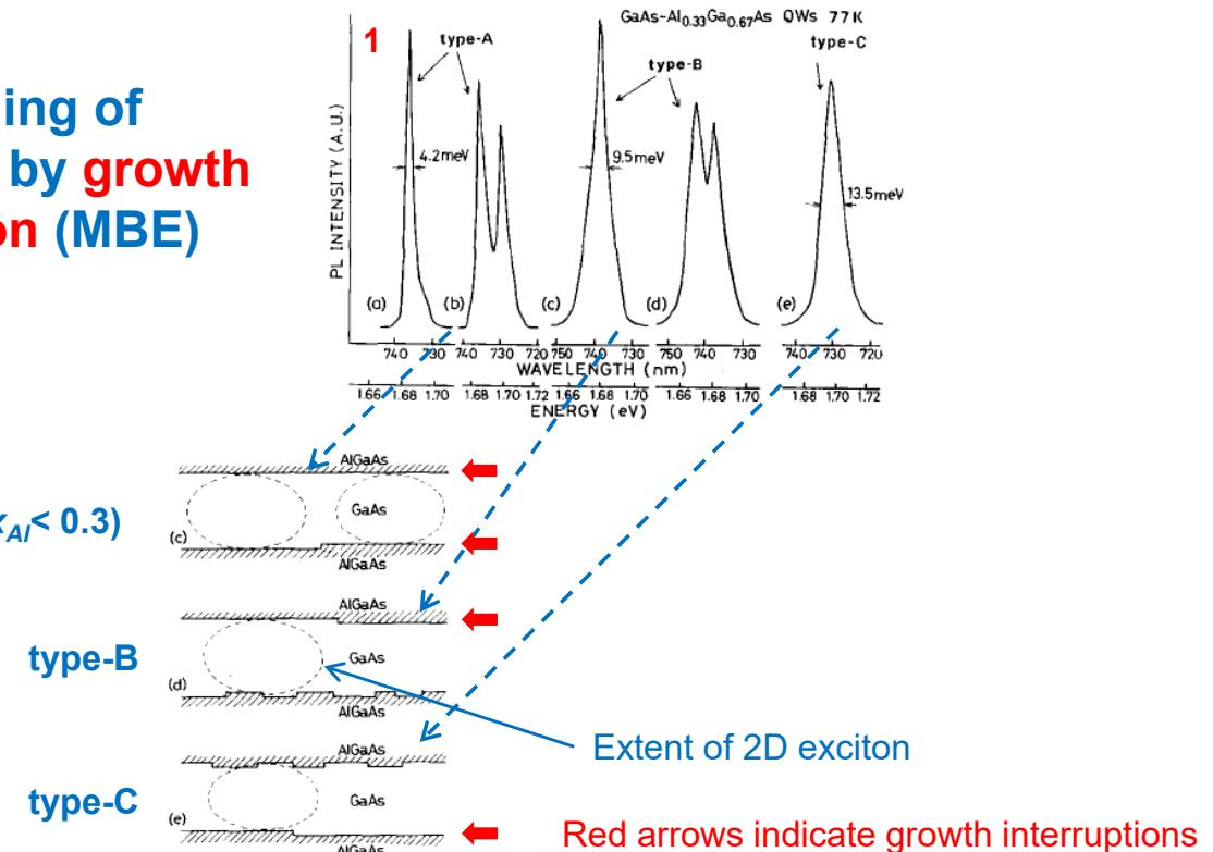
QW thickness fluctuations responsible for inhomogeneous broadening (= extrinsic broadening due to disorder)
