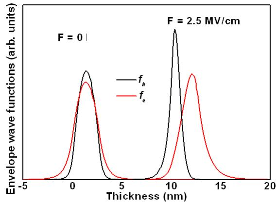
(2) spatial separation of electron and hole wavefunctions
