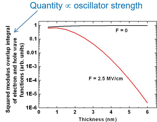
(3) decrease in oscillator strength of optical transition and exciton binding energy and
