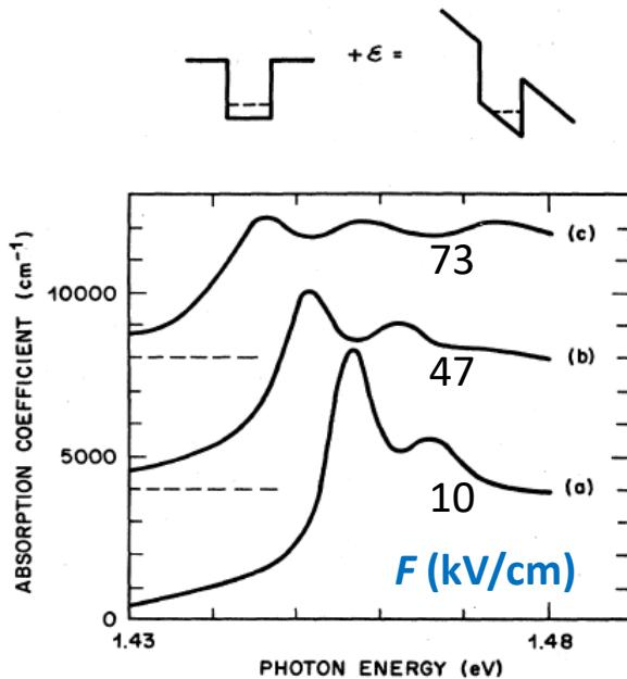
GaAs/Al<sub>0.32</sub>Ga<sub>0.68</sub>As MQWs in a *p-i-n* junction
